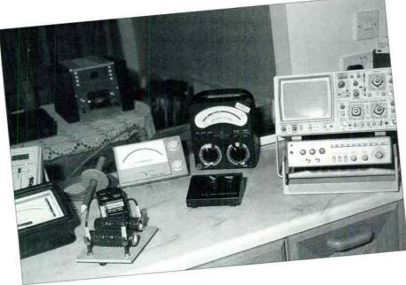
Trying to build your own amplifiers is impossible without proper test equipment. To the far right is an audio frequency generator sitting below an oscilloscope. Next to these is an Avo multi-meter, with a High Tension voltmeter to the left (used for setting up Quad ESL 57s and 63s). At the rear left is a digital multi-meter behind an analogue current meter and two high-power resistors for testing power amp output levels.
