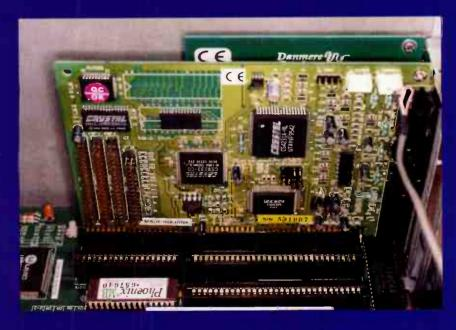
The soundcard fits into one of your PC's expansion slots. Connections provided are Line
