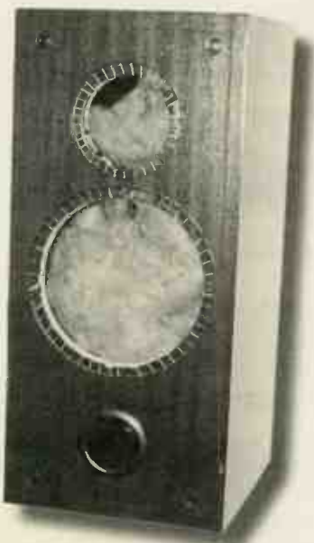
The Fablon should be applied and cut to shape before the drive units are screwed into their rebated holes.
