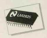
you're looking for. They now stock the new £7.50 LM2825 from National Semiconductor, which contains a complete IA switching regulator on a single chip - all you need to add for a 5v or 3.3v output is a 7-40v input. Also available is a variety of regulators from Melcher's IMR6 range, concentrating mainly on 5v and 12v supplies with prices starting at £28.69.
