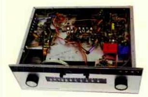
Like all electronic products of the time, the Troughline was hardwired, using discrete components. Many, like high value resistors, become noisy or fail.
