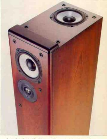
Each of the Harlech's 130mm mid/bass units is loaded with its own quarter-wave horn. The tuning frequency is at 54Hz for the front driver and 78Hz for the top one.
