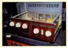
A mono Tannoy valve integrated, probably an AP30, which was a 30watt professional amplifier built during the late 50s.
