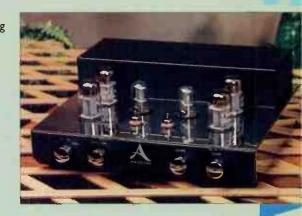
boasts the use of military spec valves. These include the input's 5814s, the 6SN7s in the driver stage and the Russian 5881s at its output. 4 and 8 ohm 'speaker taps are provided and the sockets and 'speaker terminals themselves are gold-plated.
