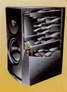
broken up by this Prism system on the back wall. Instead of a strong reflection off the rear of the cabinet being able to set up standing waves which cause colouration, the energy is dispersed, making it easier for the internal wadding to absorb. This rear surface is made from moulded plastic, with six struts linking front and rear baffles firmly together, which also helps to improve cabinet rigidity.
