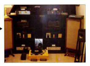
Other interesting new products included Concert Corner's "Quadrostatic" loudspeaker system, based on original Quad ESLs, with a quarter wave bass system actively crossed over at 120Hz. The original idea was by Michael Furmedge at Concert Corner, although the design work was undertaken by Colin Walker - with P. J. Walkers blessing. Keswick Audio Research showed their new Figaro Evolution and Amber loudspeakers, which fit in above existing models. They also had a prototype semi-omni directional
