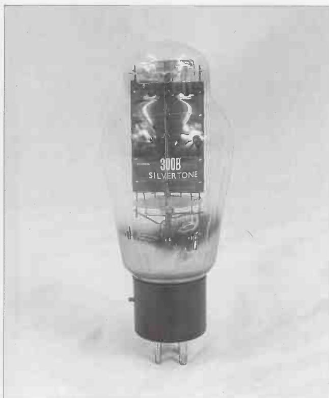
Modern production 300B valves have a lifetime of around 10,000 hours when used in a well designed circuit.
