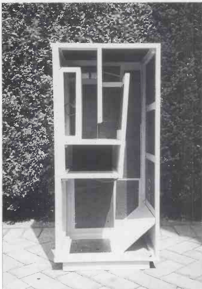
David Constant from Solihull built a version of the Cambridge R50s. This side view shows the complex internal construction.
