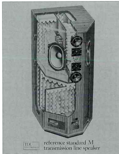
This cut-away of TDL's Reference Standard transmission line speaker shows the task a power amplifier faces when asked to drive a high power monitor. A large bass unit on either side, each rear-loaded by its own transmission line, must be driven and kept under control. At each end of the central drive unit array lies a midrange driver, both back-loaded by another transmission line. Two tweeters and one central super-tweeter complete the line-up of seven drive units.
