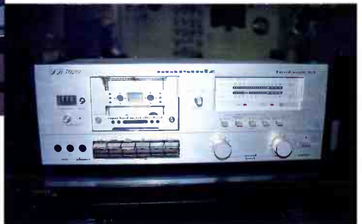
A Marantz cassette deck just in and awaiting service. This SD3020 must be one of earliest decks to have a double speed transport.
