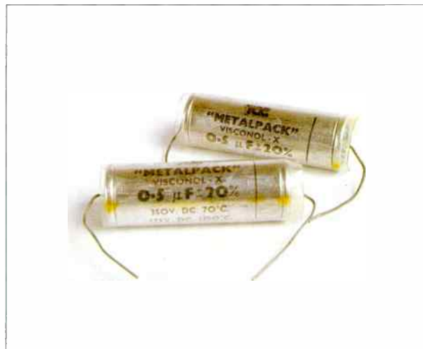
TCC paper in oil signal capacitors; these are military surplus.
