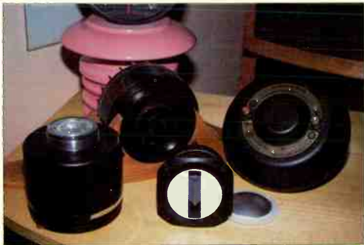
A selection of the drive units used by Living Voice. From left to right: 1. Vitavox S2 motor with a 2 inch aluminium diaphragm. 2. The Gauss tweeter used in the Air Partner. 3. Beyma CP21F slot tweeter. 4. The S5 motor unit used in the Tone Scout (nicknamed the "Landmine").
