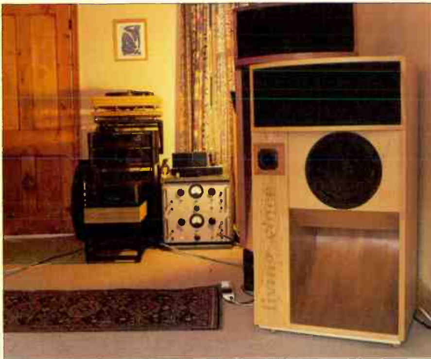
Kevin's system sits at the back behind the 'speakers. Note the two massive Solartron SRS 152 power supplies used to supply the HT voltage to the First Audio power amplifiers.
