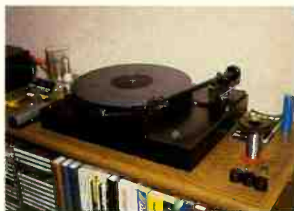
Geoff Hill's Townshend Rock turntable with silicon fluid damping trough for the tonearm.
