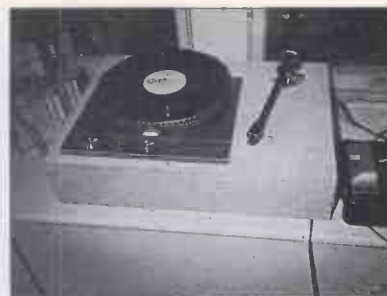
Above: Noel's Garrard 401, newly-mounted in its plinth with SME312 arm before veneering.
