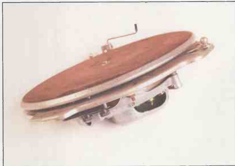
Garrard's heavy-duty 201 player from the early Thirties, designed for reproducing 78s in broadcasting and recording studios. Direct drive was used, plus a mechanical speed governor.
