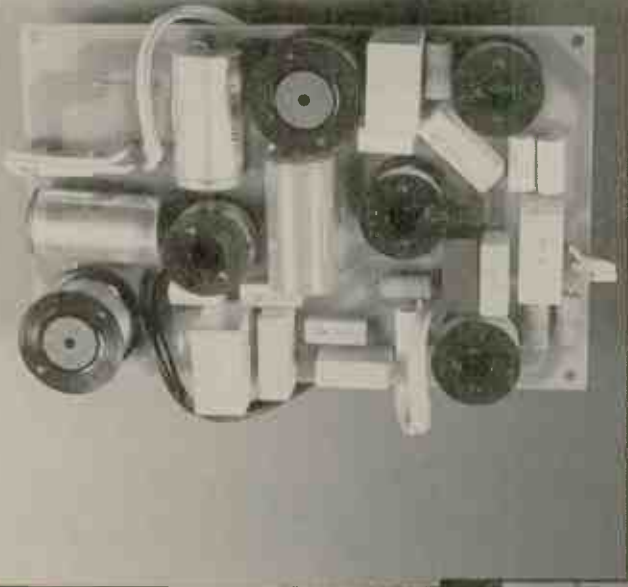
The crossover comes built. As the picture shows, it contains a large number of components. See the schematic diagram further on to identify components.
