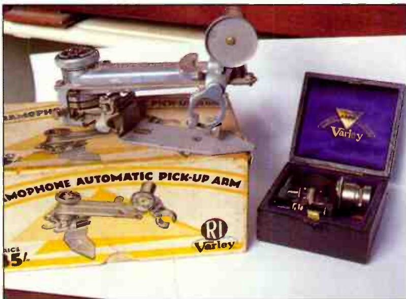
"This is an early articulated tonearm from R I Varley. It gives lovely lightweight, spring-loaded, parallel tracking; it only puts one-quarter pound (113 gms) on a record! With a sharp-ish needle they gave a cheerful sound."
