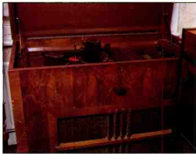
"A Gecophone made in Sept 1922 in time for broadcasting by the BBC from November 1922. Every set had to have a BBC stamp on it to show that it was approved by the Postmaster General. It would drive a pair of earphones, but it also stood on a simple amplifier that drove a small horn loudspeaker. It was disguised in a smokers' cabinet because everybody smoked in those days."
