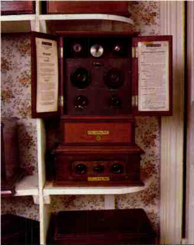
"A Gecophone made in Sept 1922 in time for broadcasting by the BBC from November 1922. Every set had to have a BBC stamp on it to show that it was approved by the Postmaster General. It would drive a pair of earphones, but it also stood on a simple amplifier that drove a small horn loudspeaker. It was disguised in a smokers' cabinet because everybody smoked in those days."
