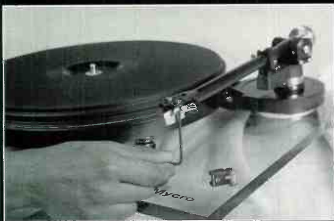
1) Loosen cartridge mounting screws just enough to allow it to slide forward or backward.
