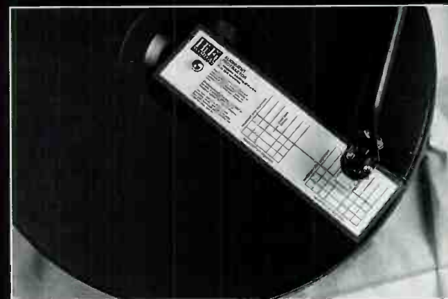
6) You can now check arm geometry by placing stylus on 'outer zero'. The side of the headshell parallel to the cartridge axis should also be parallel to the alignment lines.
