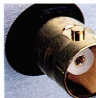
Electrical digital signals get into the DAC64 via the BNC connector (above) or an XLR socket. But analogue connections travel via the phono route (top).
