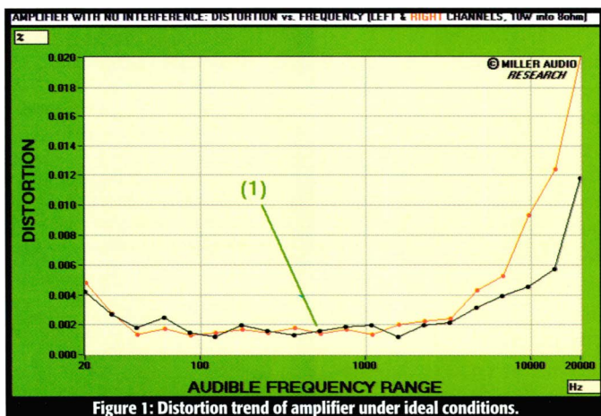
Figure 1: Distortion trend of amplifier under ideal conditions.
