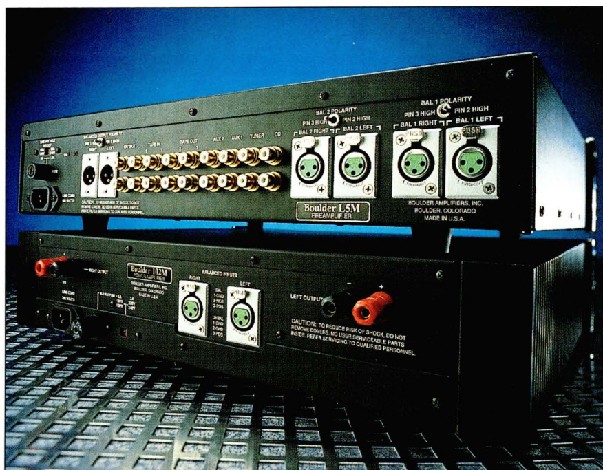
Both balanced and single-ended signals will find a warm welcome on the Boulder's back panel.
