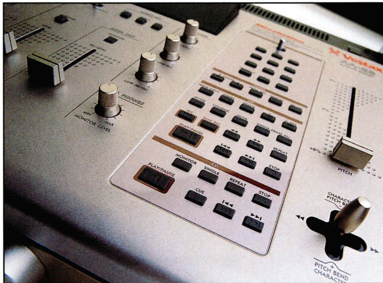
Vestax's AA-88 system has a CD player, MD recorder, FM tuner and phono inputs. Note finger-friendly joystick for the ultimate in 'digital' manipulation!
