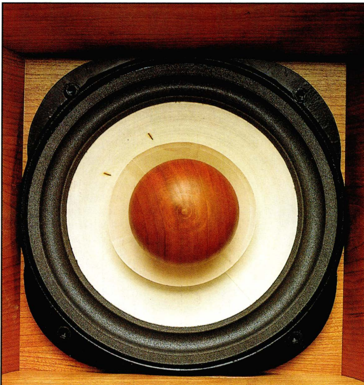
The drive-unit in the Virtuoso Gold is the Lowther PM2C. This is a full-range unit, so it does not employ a dividing network. The solid cherry-wood bulb (pictured centre) acts as a dispersion modifier.
