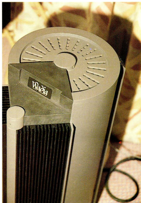
Wadia's Power DAC. A convertor with an output of 150W into 8ohms!
