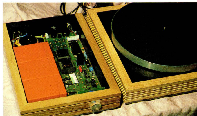
Hard cell - Pink Triangle's battery power supply is certainly speaking the right lingo.
