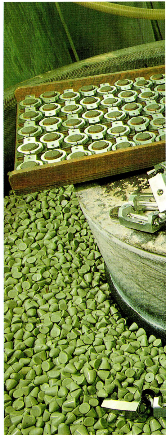
Rumblearm: Bearing yokes for Series IV, V and 300 arms being rumble finished in a drum of silicon chips.
