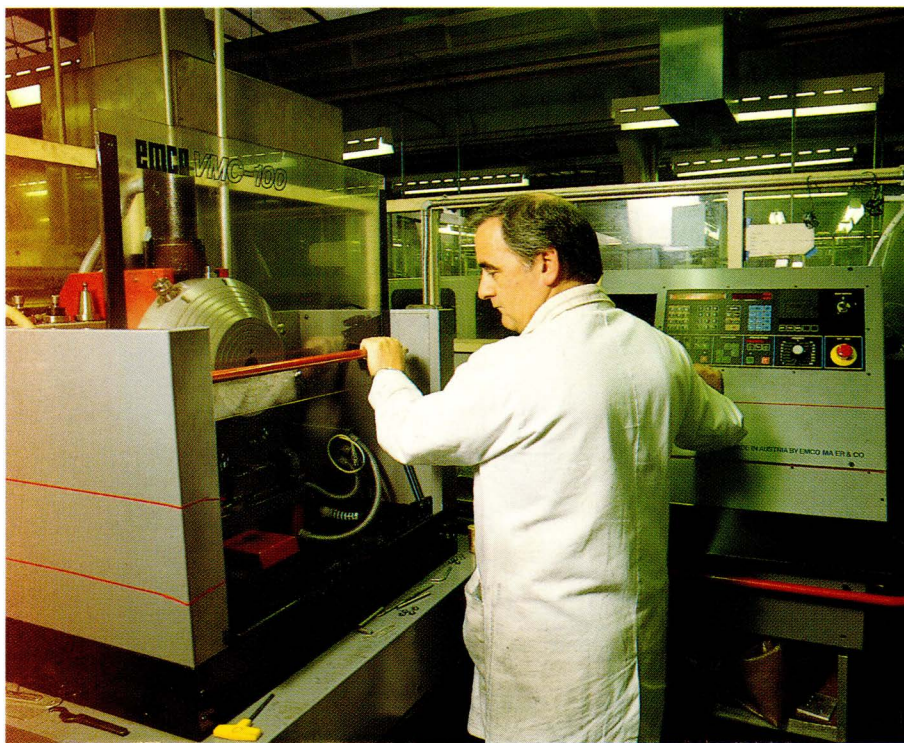
A CNC lathe in action, one of SME's engineers turns up a part for the turntable.
