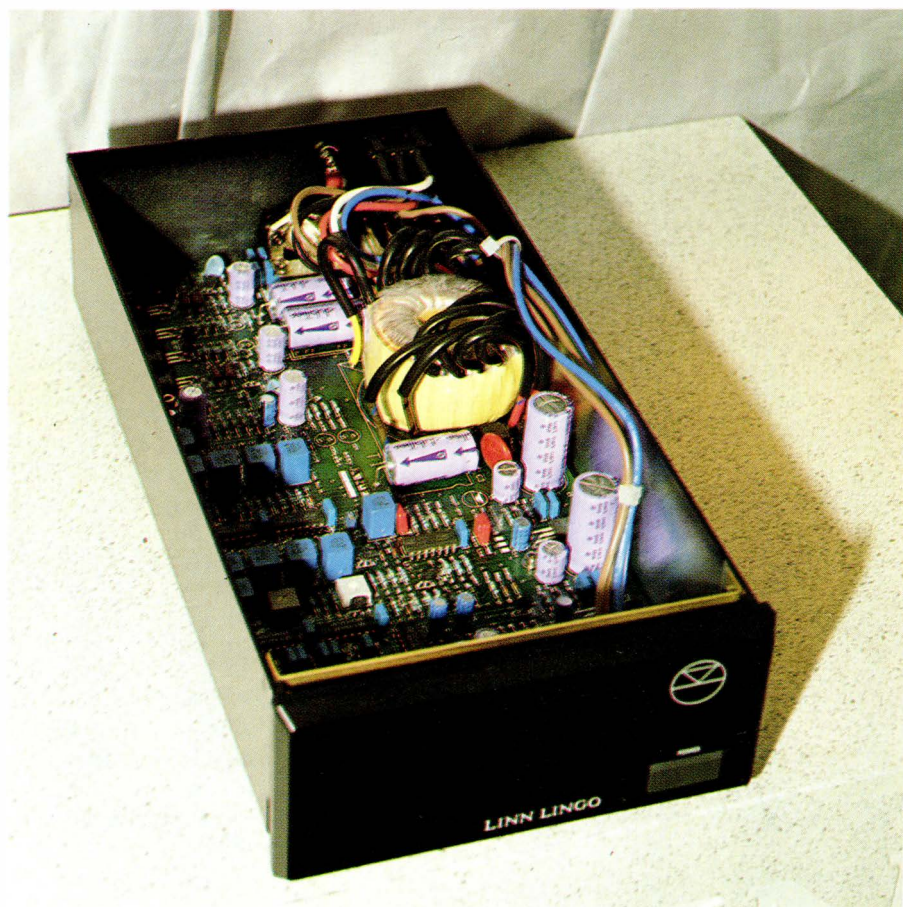
After all these years the LP12 now revolves at 45rpm, courtesy of Linn's Lingo psu.
