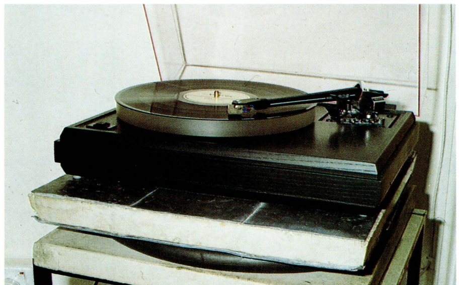
DIY turntable support – the things you can do with a car tyre inner-tube!
