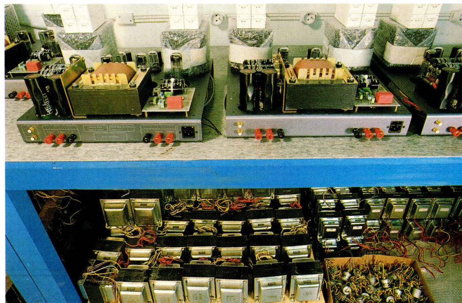
The finished product sits above a batch of (British) Partridge transformers.
