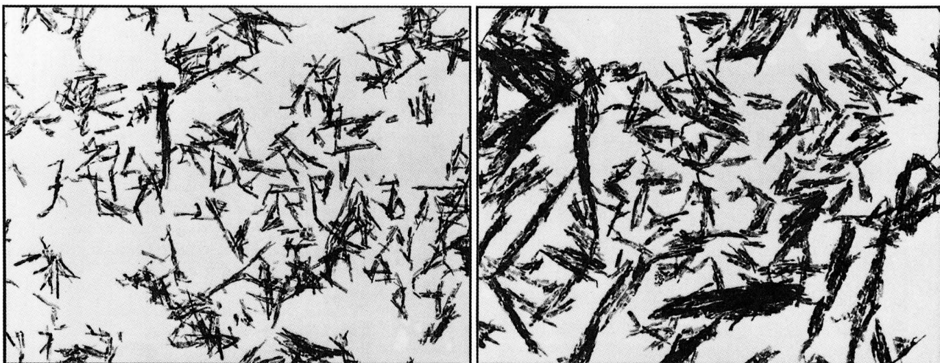
High magnification shows the difference in particle density between DAT tape (left) and a Type IV cassette (right).
