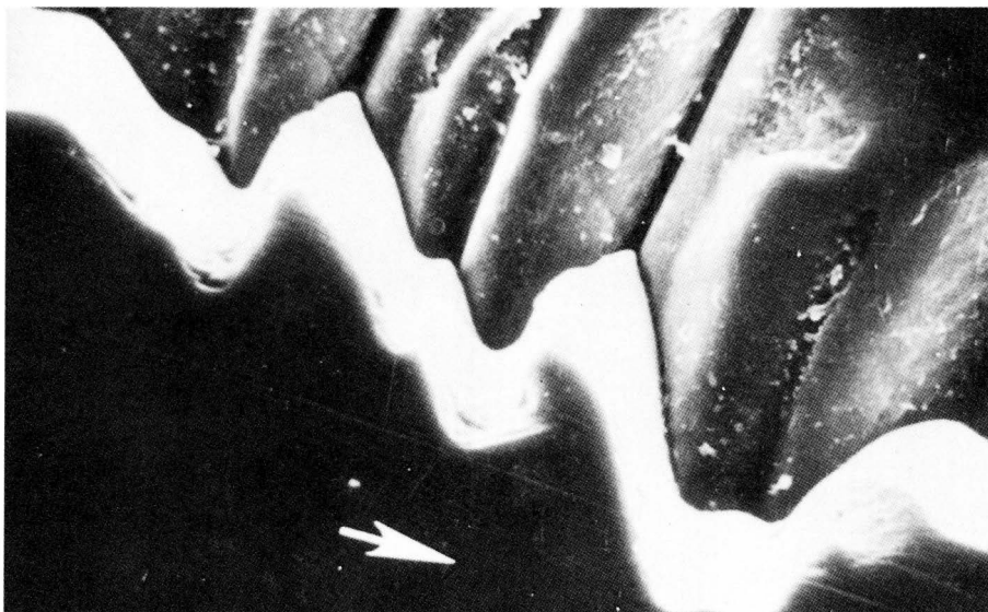
An electron micrograph shows the complexity of an LP groove.
