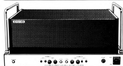
SC 25 AND STA 25 PRE AND POWER AMPLIFIERS
