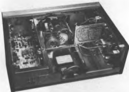
Interior of B215, showing modular electronics
