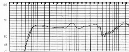
Reference sine wave response (1m on axis, 2.83V input shows sensitivity). Dashing corrects for chamber LF, dotting shows response without grill.
