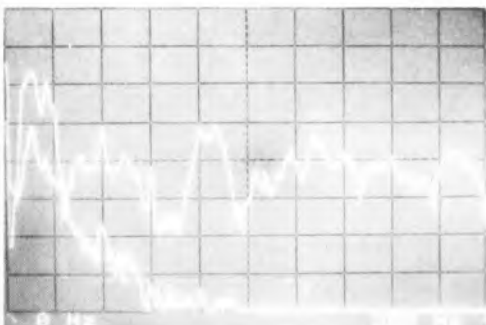
Breakthrough (0-500Hz lin): above, acoustic; below, vibration.
