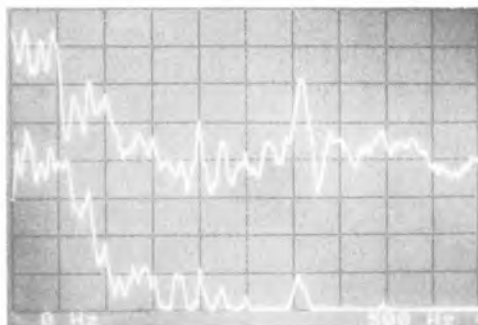
Breakthrough (0-500Hz lin): above, acoustic; below, vibration.
