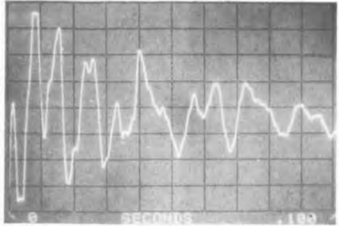
Disc impulse transmission, magnified X10.
