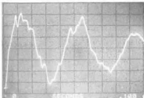
Disc impulse transmission, magnified X10.
