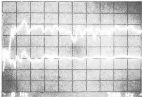
Breakthrough calibration signals: above soundfield (acoustic); below, acceleration (platform vibration) (1in freq; log amp).
