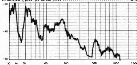
Acoustic breakthrough (microphony) of system (0dB = approx. 10 cm/s RMS, DIN rumble level, equivalent to loud music output from turntable).
