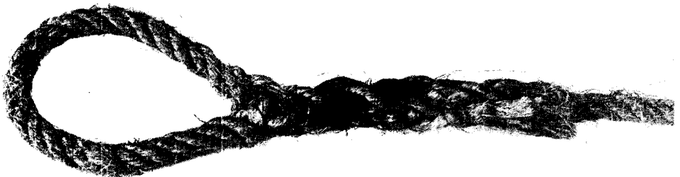
HOW AN EYE IS MADE IN A ROPE BY SPLICING
