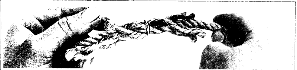
Fig. 5. Both ends of the unlaied rope are being passed into the standing portions to make the splice; the ends of the strands are still loose at this stage
