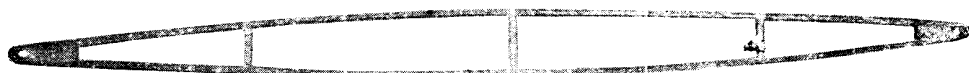
Fig. 2. Constructed of two main members and fitted with distance pieces this spreader has a very distinctive appearance, and is very light considering its strength
