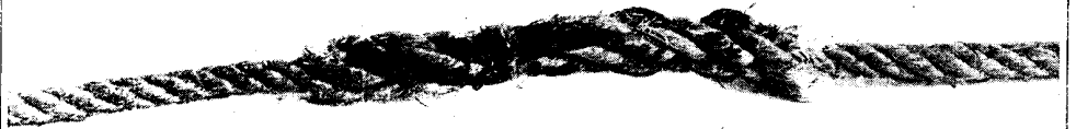
Fig. 6. In this photograph the short splice is complete, but left loose to show how the strands are placed. When the rope is pulled tight the loose ends are trimmed off
