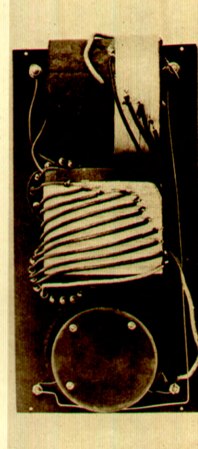
Fig. 19. This is a view of the back of the panel of the complete loose coupler showing the coils with their tapplings and the condenser.
