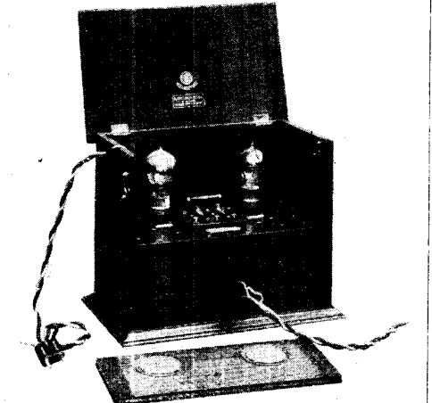
Fig. 6. By means of a switching device, either one or two stages of low frequency may be employed in this Marconiphone set
