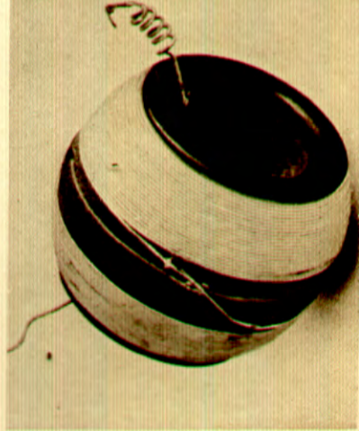
Fig. 17. Rotor used for tuning in short wave-lengths shown complete.
