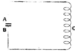
Fig. 59. Closed oscillatory circuit used for setting up a train of electro-magnetic waves
