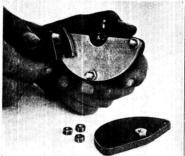
Fig. 42. Two fixed plates are attached to the ebonite top. These are mounted on three upright posts and kept in position by spacers and nuts. The bottom ebonite plate is added when the movable part is attached
