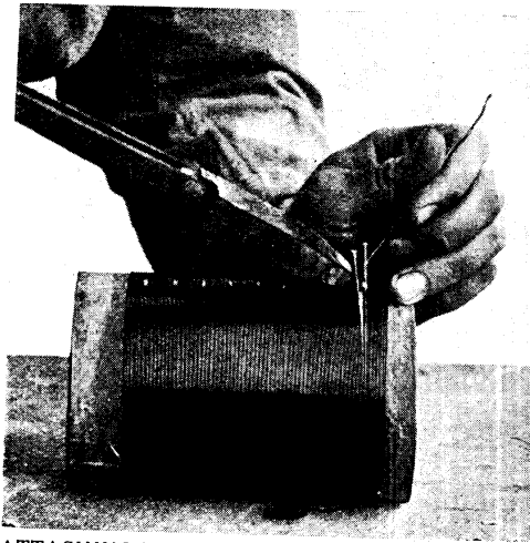
Fig. 23. Tappings are made by soldering leads to the coil at specified numbers of turns of wire. At the turn which is to be tapped the single wire is isolated by means of pins, and the lead soldered on as shown in the photograph
