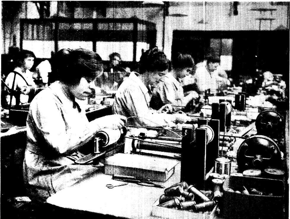
COIL WINDING ON A LARGE SCALE AT THE MARCONI WORKS
