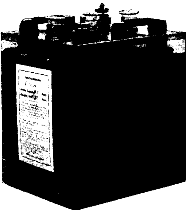
Fig. 3. This 6-volt accumulator has five plates per cell and capacity of 20 ampere-hours for filament heating
