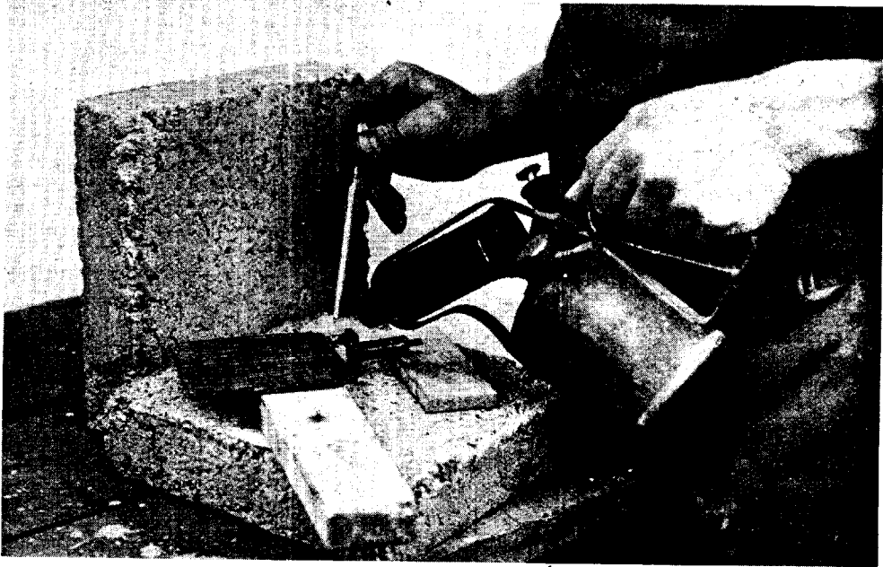
Fig. 24. Plate being fitted with new lugs by lead burning. The plate is supported on breeze blocks to retain the heat and prevent the surface of the bench from being burnt
