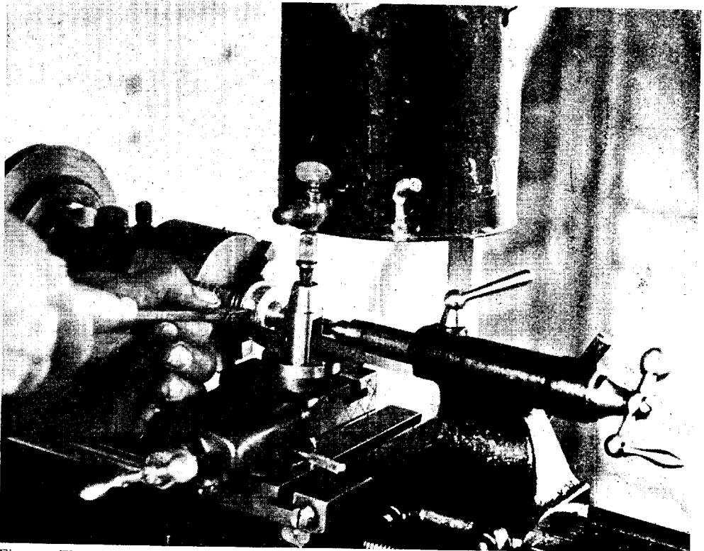
Fig. 1. The correct arrangement for lubricating the tool when turning aluminium provides for the lubricant to be directed to the point of the tool
