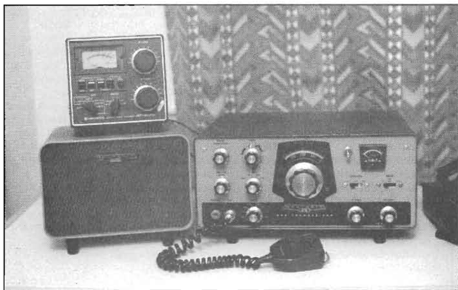
The HW-100, belonging to G0GGV, and SB-600 speaker with HP-23 PSU inside
