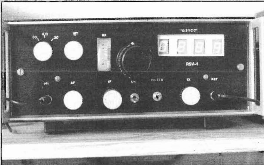
G3YCC's homebrew 80/40/20m transceiver
