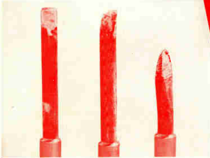
The bit on the left, used with Savbit Alloy, has made 10,000 joints. The centre bit, used for 1,000 joints, and the bit on the right for 7,500 joints, were used with a standard tin/lead alloy.
