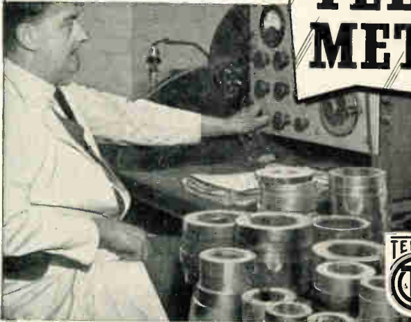
Routine Factory testing of Mumetal toroidal cores.
