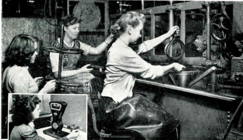
Testing at every stage. Infinite care is taken to maintain high quality of cones. (Left) 'Felts' from the drying oven are tested visually for texture before being weighed on a delicate balance.
