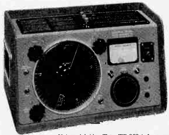
Universal bridge Type TF 868A for measuring inductance 1\mu H - 100H , capacitance 1 pF - 100 \mu F , resistance 0.1 \Omega - 10 M\Omega . A bridge-voltage monitoring system is incorporated. (Marconi Instruments Ltd.)
