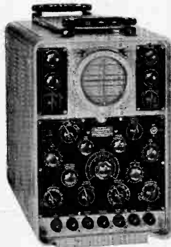
Model 1059 double-beam wideband oscilloscope. The instrument has two similar amplifiers and a 4-in. p.d.a. tube. The sensitivity of the calibrated amplifiers is continuously-variable between 0.1 V/cm to 10 V/cm over a working bandwidth of 5 c/s to 10 Mc/s but additional pre-amplifiers covering the range 10 c/s-200 kc/s are provided. (Cossor Instruments Ltd.)
