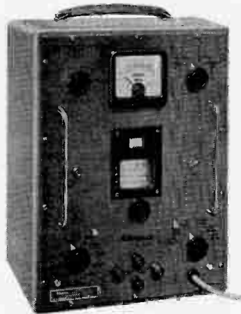
Low-frequency signal generator covering 15 c/s-200 kc/s. Output: 35 dBm to +25 dBm in 600 ohms, frequency stability 0.1% at 1 kc/s, harmonics and hum -40 dB when the output is 1 mW. (Advance Components Ltd.)
