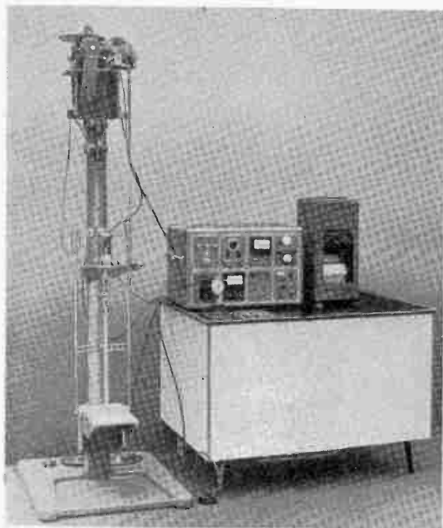
Dynamometer for extensile testing. (Research Association of British Rubber Manufacturers)
