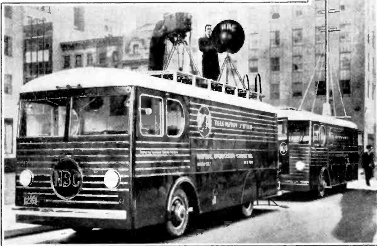
Two vans are used in America by the National Broadcasting Company for experimental television outside broadcasts and are connected by a coaxial cable. One van contains a transmitter with a "trolley" aerial, and the other the camera equipment with the necessary cameras and microphones.
