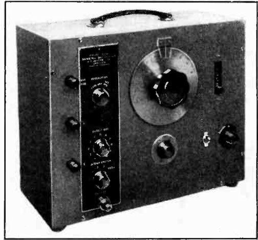
Cossor Model 3343 ganging oscillator.
