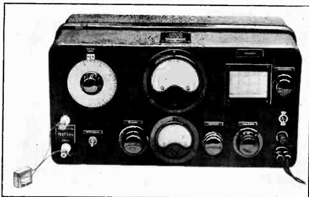
Salford "Q" meter for measurements of coil magnification.
