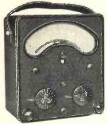
The newest multi-range Avometer, with 46 ranges.
