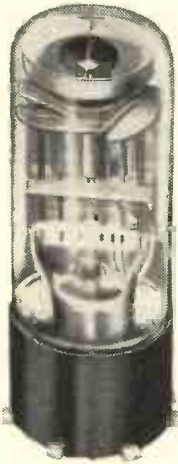
Fig. 4.—Mullard TV4 Cathode-Ray Tuning Indicator and (below) circuit in which it is used. For full brightness only 4 volts at the grid of the built-in triode amplifier is required.
