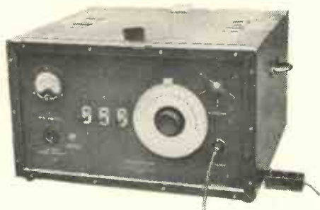
Wearite mains-driven Signal Generator, Type TD 6.
