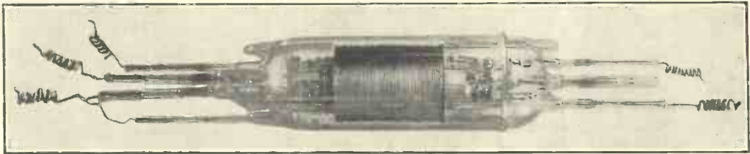
Fig. 2.—Silica Pentode constructed in H.M. Signal School, Portsmouth.
