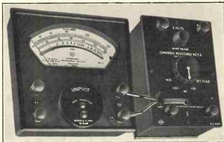
Fig. 2.—Standard "Unipivot" galvanometer with the ohmmeter coupled to it.
