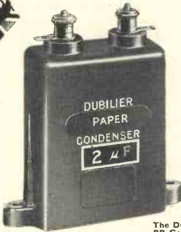
The Dubilier Type BB Condenser is a high-efficiency condenser in moulded bakelite case. Working voltage 200 D.C. (peak) Test voltage 400 D.C. Capacities from .09 mfd to 4.0 mfd. Prices from - - 1/9
