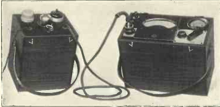
Fig. 2.—Multi-range mains operated valve voltmeter.
