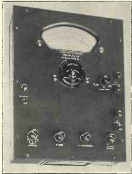
Cambridge thermionic millivoltmeter employing three stages as follows. (1) H.F. amplifier, (2) detector, (3) balancing valve.
