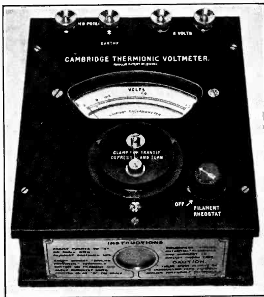
Cambridge unpivot thermionic voltmeter.
