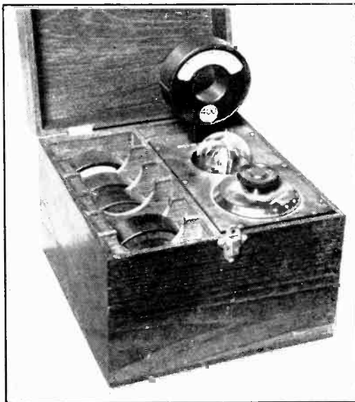
Dubilier Wavemeter, in which the glowing of a neon lamp indicates resonance.
